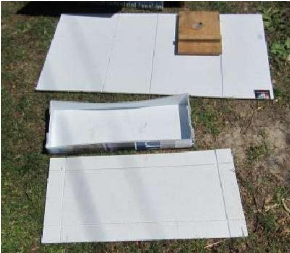
These measurements are a little rough as I just use an old cut out as a template when I want to make more rather than re-measure everything again. The timber ends are 7 1/8 x 11 1/16 x
